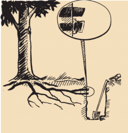
Figure 26. When digging near trees suitable for preservation, the first cut should be made by hand labor with shovels under supervision of an arborist. Exposed roots should be neatly cut with a sharp saw. To protect them from drying out, the ends of severed roots can be covered with a plastic sandwich bag held in place by a rubber band.
