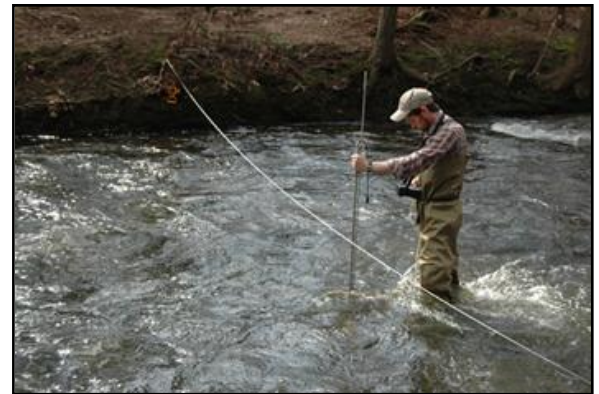
Mike Yanchuk, DCCD Watershed Specialist, measuring the flow of Clarks Creek
